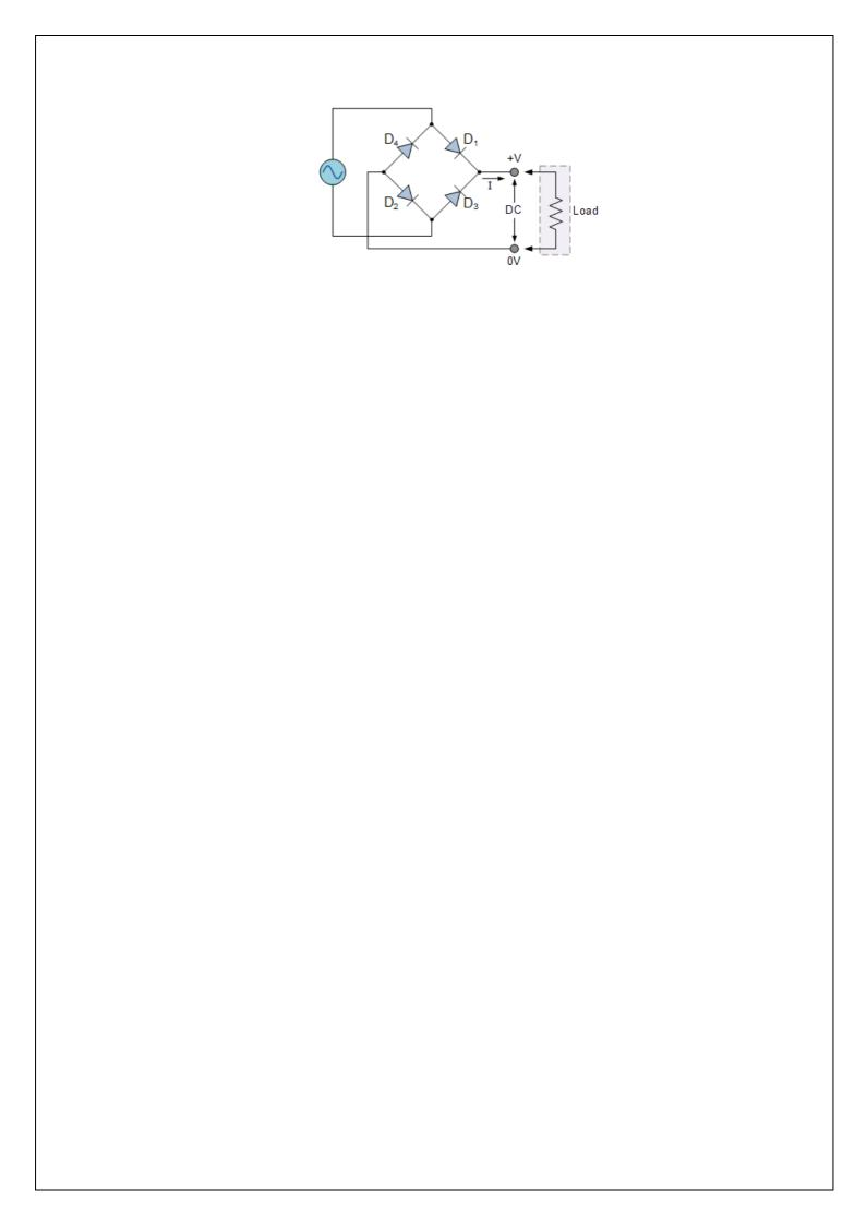
During the positive half cycle of the supply, diodes D1 and D2 conduct in series while diodes D3 and D4
