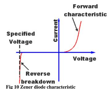
Although the voltage reference diode is normally referred to as a Zener diode, there are two different breakdown mechanisms that can occur:
