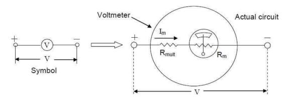
Using the same meter movement, a multirange voltmeter can be designed. A three-range Voltmeter
