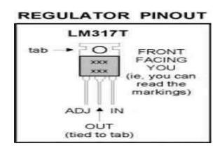
$Pin-1 \ adjustable/variable \ , \qquad Pin-2 \ V_{out} \& \qquad \qquad Pin-3 \ V_{in}$
