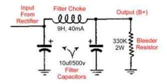
In this filter one inductor & two capacitors are used.
