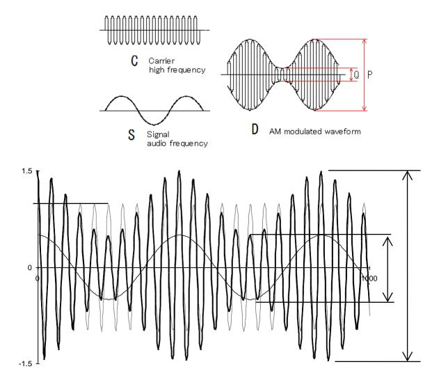
Figure 1.2 An AM signal with modulating and carrier signals shown
