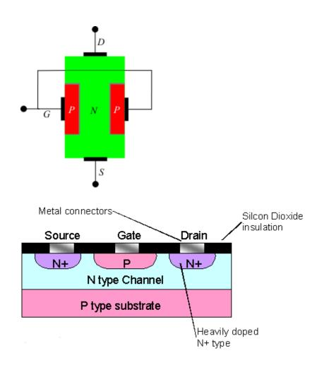
The JFET operates on the principle that channel width and hence resistance of the conducting channel can be varied by changing the reverse voltage between gate to source ( $V_{GS}$ ).
