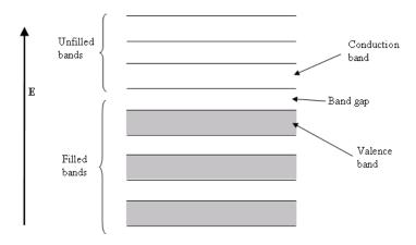
Fig 1. Energy band diagram
