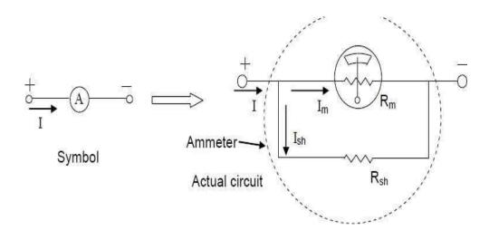
A given meter movement can be used to build a multirange ammeter. Each range requires a different value of the shunt resistance. So a three-range ammeter requires three different shunt resistors.
