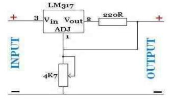
By varying the value of  $R_2$ the output voltage can be adjusted.
