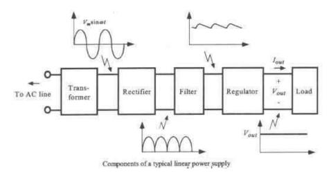
Working Principle: The output of power supply  $(V_{in})$  is fed to the voltage regulator which produces the final output  $(V_{laod})$ . The output voltage  $(V_{laod})$  remains constant whether the load current changes or there are fluctuations in the AC input.
