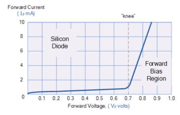
The application of a forward biasing voltage on the junction diode results
