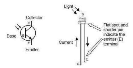
Working Principle: The electrons that are generated by photons in the base-collector junction are injected into the base, and this photodiode current is amplified by the transistor's current gain  $\beta$ . If the emitter is left unconnected, the phototransistor becomes a photodiode.
