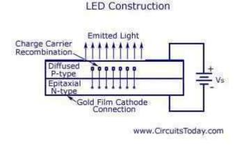
Fig. LED Construction
