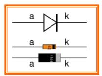
Small **signal diodes** can be damaged by heat when soldering, but the risk is small unless you are using a **germanium diode** (codes beginning OA...) in which case you should use a heat sink clipped to the lead between the joint and the diode body. A standard crocodile clip can be used as a heat sink.
