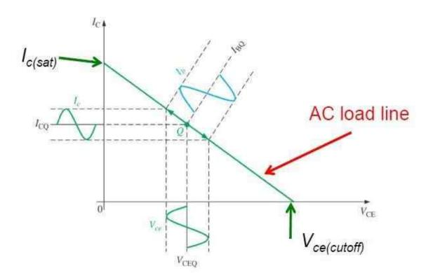
$$V_{CE max} = V_{CE} + I_C R_{AC}$$
