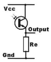
Common collector / emitter follower phototransistor circuit
