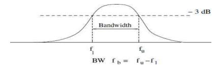
**Where**  $f_u$  is the upper cut-off frequency and  $f_l$  is the lower cut-off frequency.
