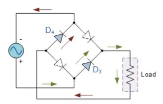
Max. rectifier Efficiency= Max. d.c.output power/ a.c. input power= $\dot{\eta}$  =81.2 %
