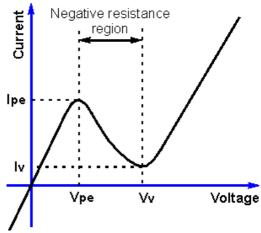
Fig 14 Tunnel diode VI characteristic
