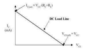
ii) When transistor is off  $I_{c(Sat)}=V_{CC}/I_{c(Sat)}$
