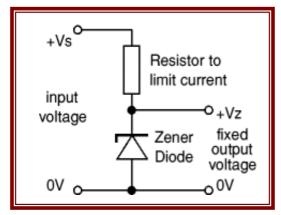
Fig 12 Simple circuit of a Zener diode shunt regulator
