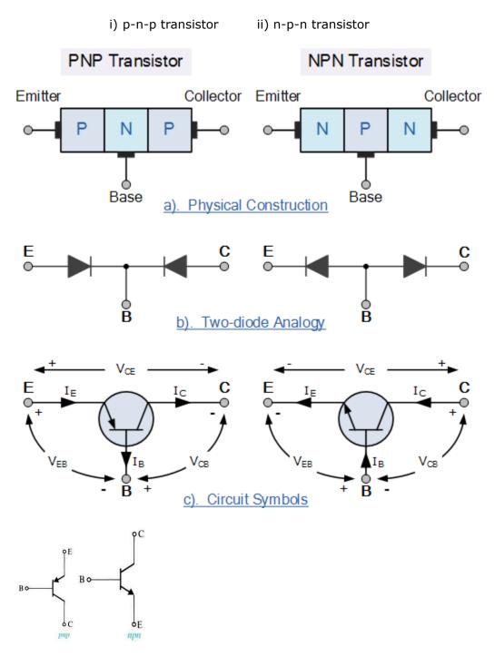
The direction of emitter arrow indicates direction of current flow.
